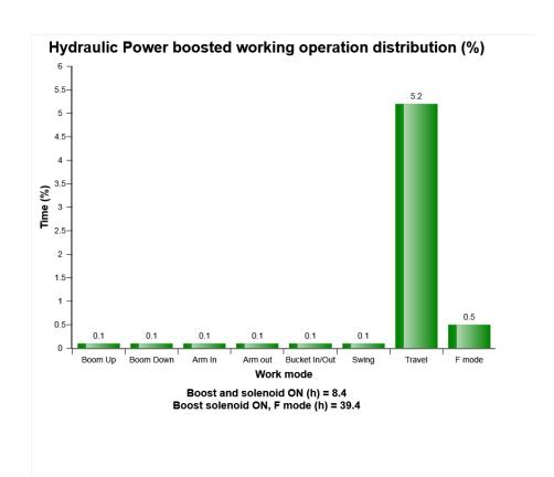
T he diagram describes Power boosted operating time distribution, when main relief pressure increases on working operation modes. In this diagram, the sum of time (%) of each working operation mode can exceed 100%. It means that customer has been operated several working operations at the same time.
