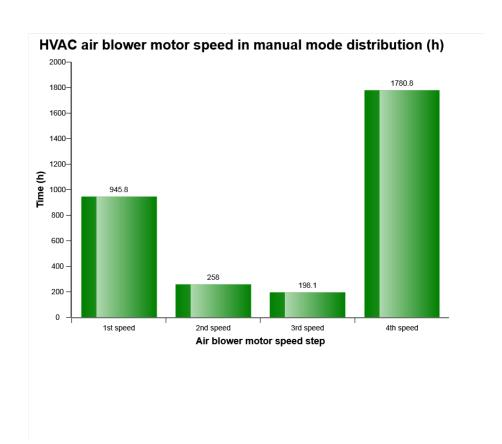
The diagram describes air blower motor speed distribution for HVAC manual control mode established by operator in Cabin.
