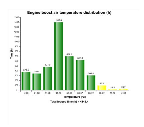
The diagram describes Engine boost air temperature distribution of the machine when the engine is
