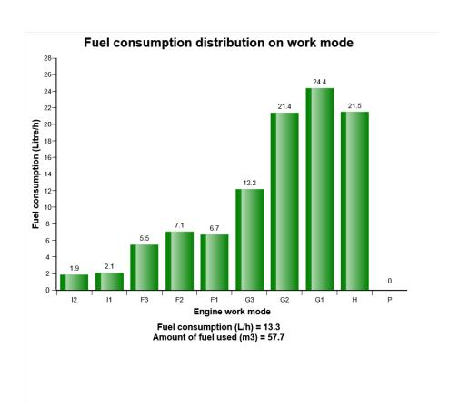
This diagram shows the fuel consumption distribution rate on each work mode.
