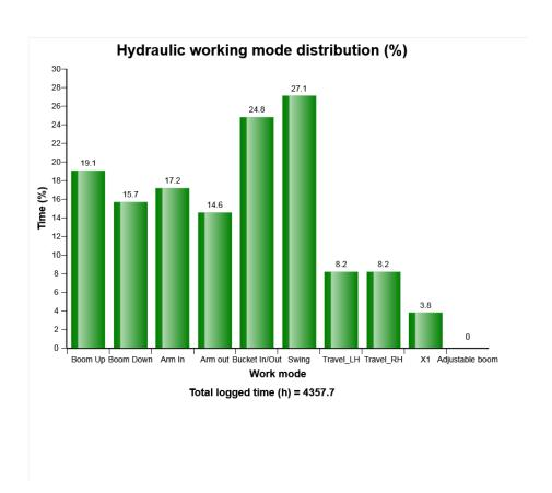
The diagram describes hydraulic working operation mode distribution.
