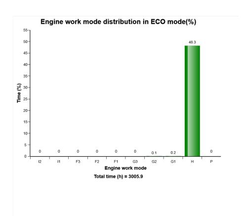
This diagram shows the distribution of the engine work mode in percentage of time when ECO mode is engaged.
